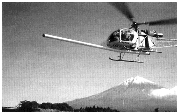
Fig. 1 Helicopter equipped with new aeromagnetic survey system with a nose boom configuration.
