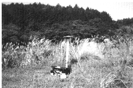
Fig. 5 GPS receiver on the ground as a reference station for the differential processing.
